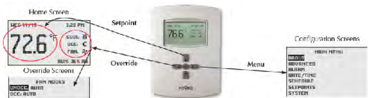
FIGURE 2 ECU Series Controller Home, Override and Configuration Screens
