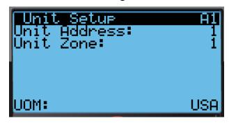
In addition to setting up the address, the user may also want to set the unit zone and unit of measure. Unit addresses can only be used once per LC6000 regardless of number of zones.
