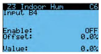
Press UP or DOWN key to change value to ON to enable sensor (or change value to OFF to disable sensor).
