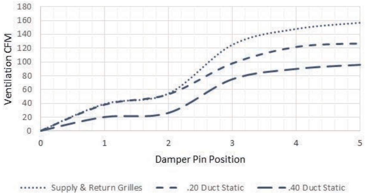
GRAPH 1 W18*B FAD-NE2, 3 W/O Exhaust Ventilation Delivery
