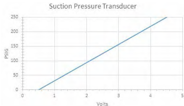
FIGURE 2 Voltage to Pressure: Suction Pressure Transducer
