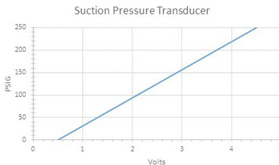
FIGURE 2 Voltage to Pressure: Suction Pressure Transducer
