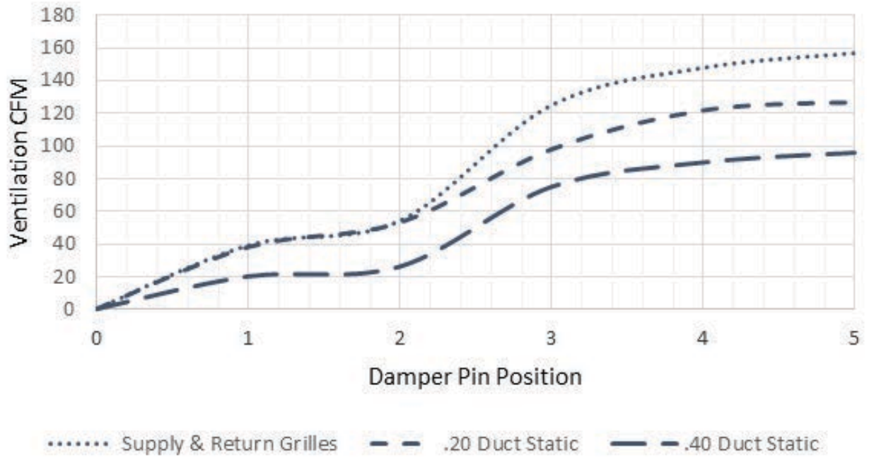
GRAPH 1 W18HB FAD-NE2, 3 W/O Exhaust Ventilation Delivery
