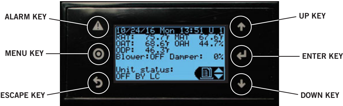
FIGURE 28 TEC-EYE (Bard P/N 8301-059) Display and Interface (Status Screen Shown)
