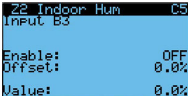
FIGURE 35 Enable/Disable Zone 2 Indoor Humidity Sensor
