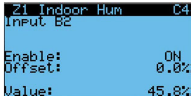
FIGURE 33 Enable/Disable Zone 1 Indoor Humidity Sensor
