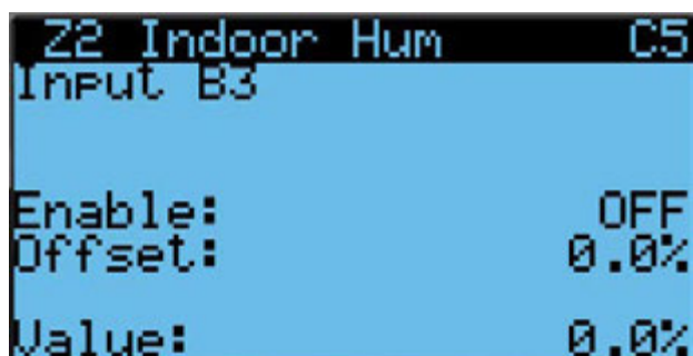
FIGURE 35 Enable/Disable Zone 2 Indoor Humidity Sensor
