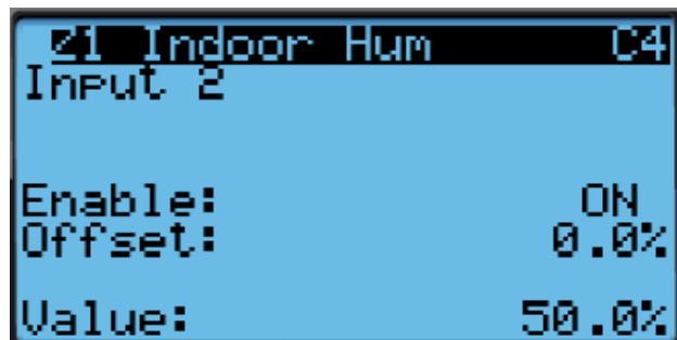
FIGURE 46 Adjusting Sensor Offset Value
