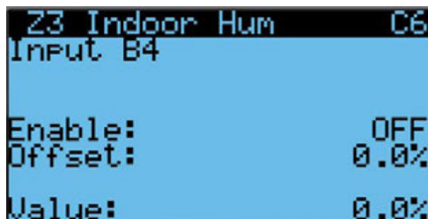
FIGURE 36 Enable/Disable Zone 3 Indoor Humidity Sensor
