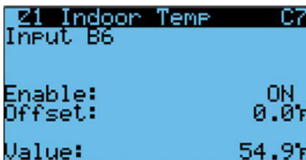
FIGURE 37 Enable/Disable Zone 1 Indoor Temperature Sensor
