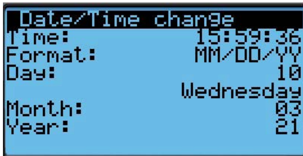
FIGURE 32 Setting Controller Date and Time
