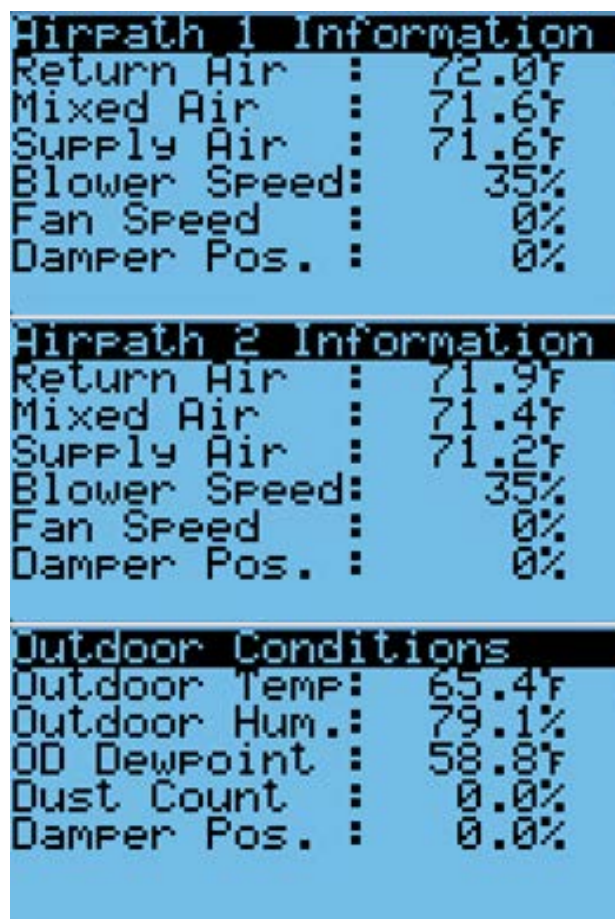
FIGURE 6 Unit Air Path Information
