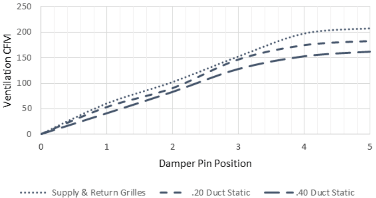
GRAPH 4 W36HY FAD-NE2, 3 W/O Exhaust Ventilation Delivery
