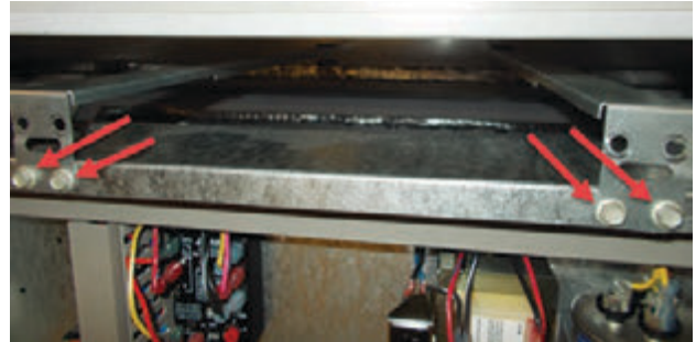
FIGURE 6 Remove Four Screws
