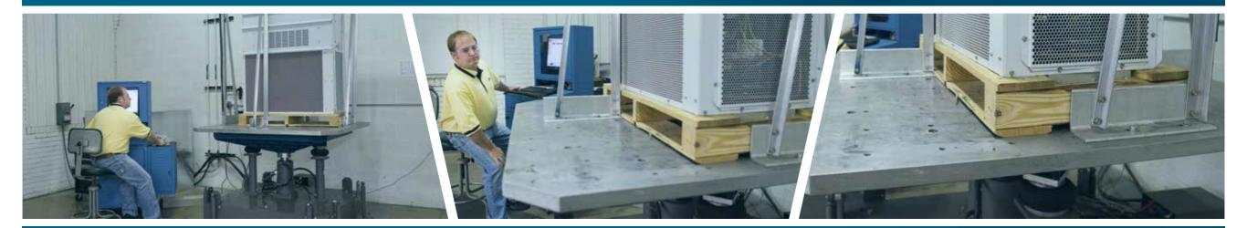
Whether traveling from the modular manufacturing site to initial location, or between locations, our units have been extensively shake tested to ensure that everything remains fully operational and right where it is meant to be.
