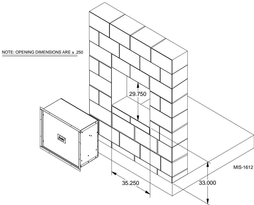
the sleeve level and square in the opening. A slope is built into the bottom of the sleeve from the inside to the outside. This will allow any water that gets into the sleeve to drain out. Once the test fitting has been checked out, the sleeve should be removed from the wall.
