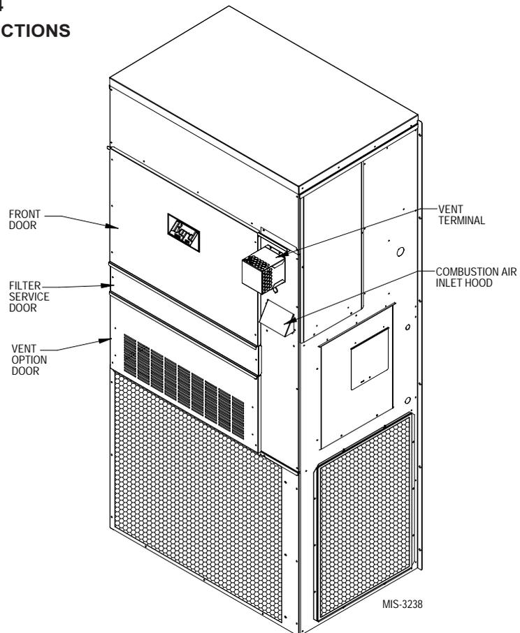
4. Inspect the vent terminal, or vent system observing for any debris from weather, birds, and the like. Clean if necessary. Also check the combustion air inlet hood to make sure it is clear. See Figure 4.
