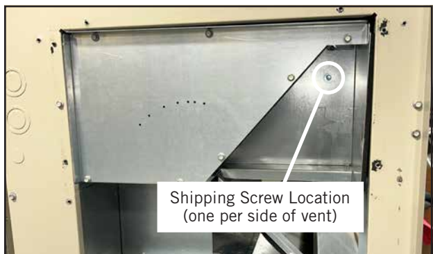
FIGURE 13 Remove Blade Shipping Screws
