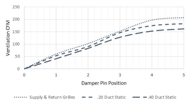
GRAPH 4 W36\*Y FAD-NE2, 3 W/O Exhaust Ventilation Delivery
