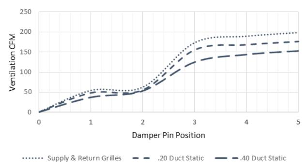
GRAPH 3 W30\*Y FAD-NE2, 3 W/O Exhaust Ventilation Delivery
