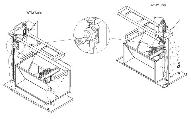
FIGURE 16 Dirty Filter Switch Location
