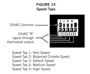
Multiple motor speed taps may be energized simultaneously by 24VAC power during different modes of operation. The highest number speed tap energized takes priority with 5 being the highest and 1 being the lowest. See Table 15 for the corresponding blower speeds with the different modes of operation.
