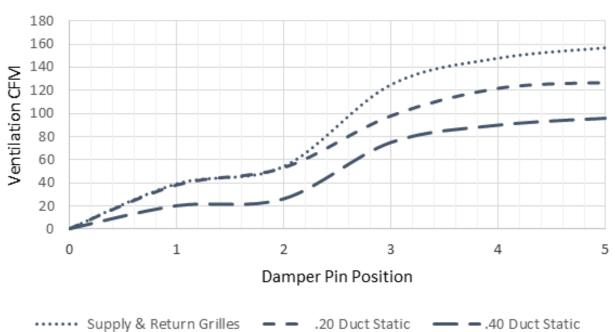
GRAPH 1 W18\*Y FAD-NE2, 3 W/O Exhaust Ventilation Delivery
