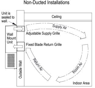
Non-ducted installations supply conditioned air into indoor room areas without extensive duct work. The supply airstream is directed by adjusting the 4-way supply grille to reach areas being conditioned. The supply air mixes with the room air and cools or heats occupants and/or equipment in the area. Unconditioned room air is returned to the unit through the return grille. Avoid supply air leaving supply grille and re-entering the unit return grille without mixing with room air.
