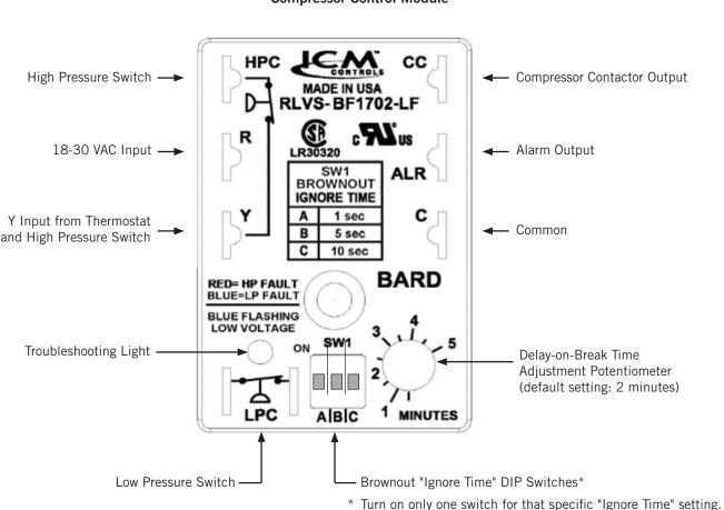
FIGURE 10 Compressor Control Module
