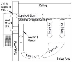
Indoor sound plenums are installed inside the room over the unit return air opening. Plenum use can provide sound isolation and indoor area sound reduction. The WAPR11 sound plenum provides a single solution for all unit tonnage sizes. The WAPR11 may be installed horizontally or vertically in the room. Unit duct static requirements cannot be exceeded when using a sound plenum. Follow all instructions provided with the sound plenum when installing the product.
