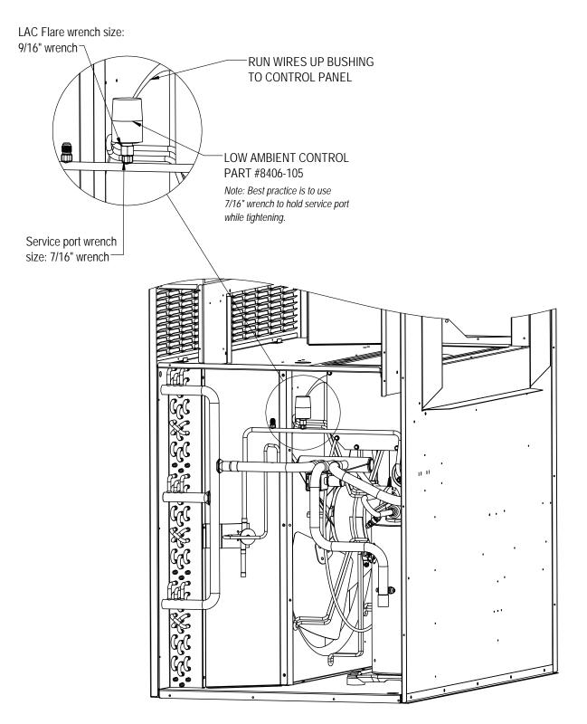
FIGURE 3 Freeze Protect Thermostat Location and Wire Routing
