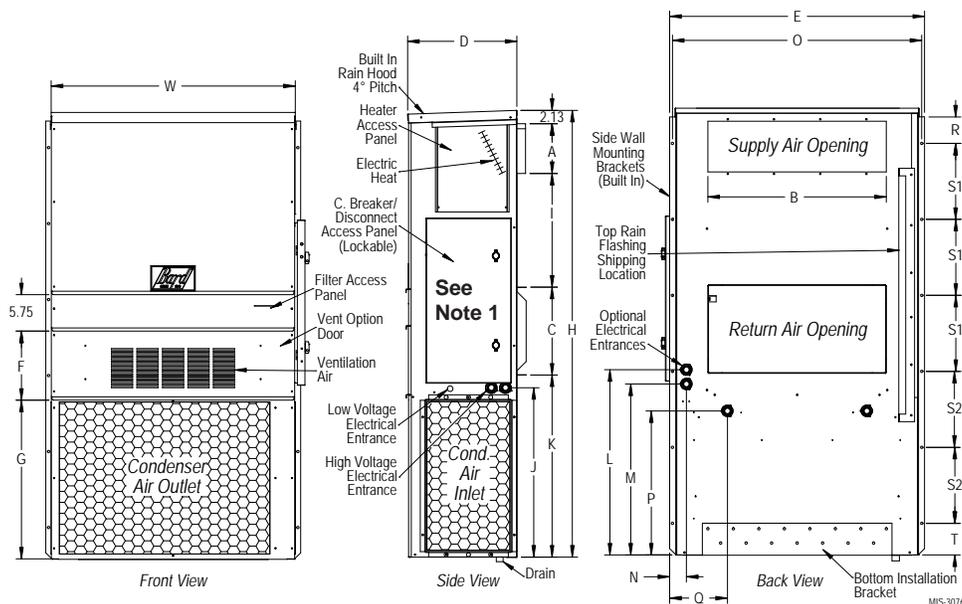
**Note 1:** Desert Duty control panel door is shown and is standard. For optional flush Moderate Duty Control Panel Cover, order Control Cover option "M". See Nomenclature on Page 8.
