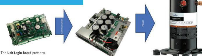
The **Unit Logic Board** provides information to the Inverter Drive including capacity needs of the indoor space. It also supplies signals to the indoor and outdoor fan motors, ventilation options, valves, and sensors.
