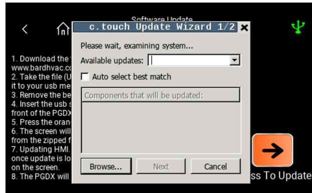
After the correct file has been placed on the memory stick, re-insert the memory stick and press the update button again. If the correct file is on the memory stick, the screen will show the "Updating HMI..." splash screen (See Figure 8).
