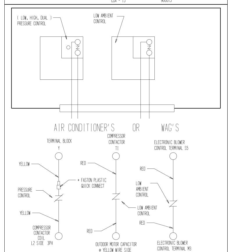
\* THIS CONNECTION MUST BE MADE WITHIN THE CONTROL ENCLOSURE.
