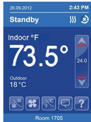
Local humidity only shows on models with the humidity sensor present and when enabled by configuration property RH Display.
