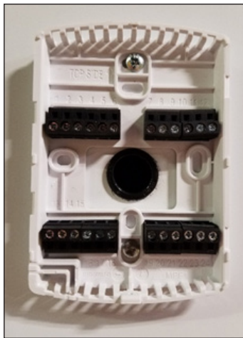
FIGURE 4 Connect Wires to Thermostat Sub-Base
