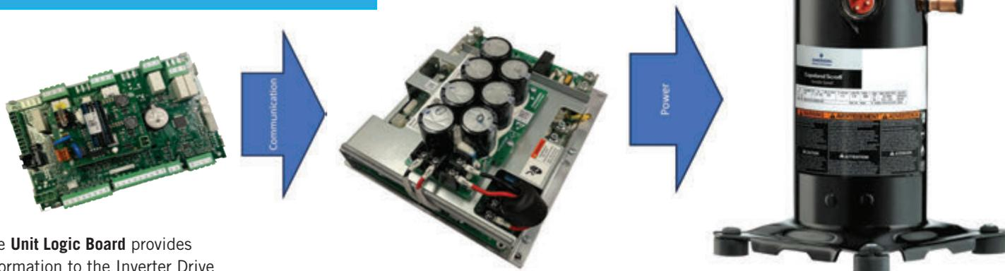
The **Unit Logic Board** provides information to the Inverter Drive including capacity needs of the indoor space. It also supplies signals to the indoor and outdoor fan motors, ventilation options, valves, and sensors.
