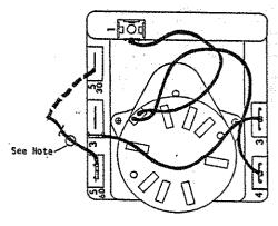
NOTE: All models are connected to 5/60 terminal (60 minute).
