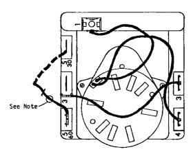
NOTE: All models are connected to 5/60 terminal (60 minute). Any model can be changed from 60 minutes to 30 minutes by unplugging from 5/60 terminal and reconnecting to 5/30 terminal as shown by dotted line.
