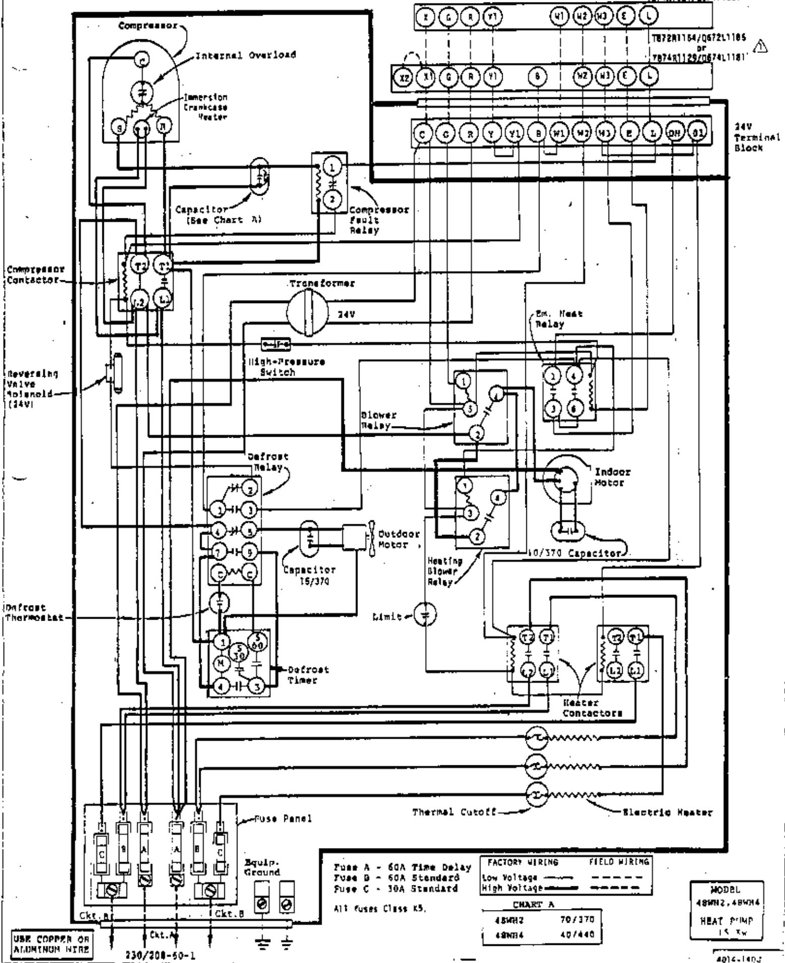
**⚠** If there is an X1 and X2 terminal on Q674L1181, jumper them together and connect from C to either one.
