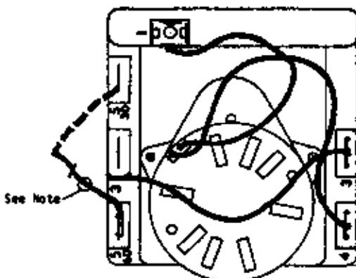
**NOTE:** All models are connected to S/60 terminal (60 minute). Any model can be changed from 60 minutes to 30 minutes by unplugging from S/60 terminal and reconnecting to S/30 terminal as shown by dotted line.
