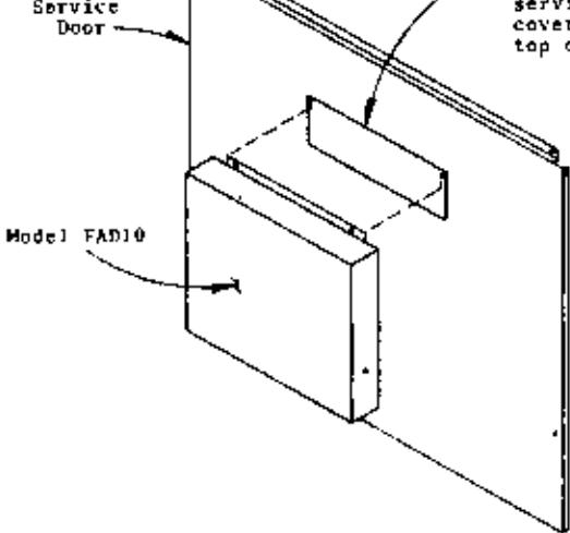
Insert top flange of fresh air cover into opening in service door and push top of cover assembly all the way to top of opening.
