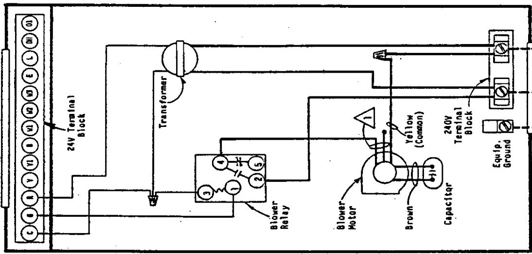
**⚠** Factor Y connected on high speed (block). Low speed not used.
