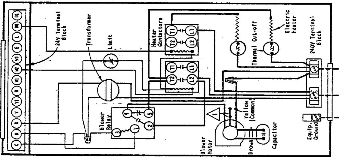
Factory connected on high speed (Black), 00 NOT use low speed (Red).
