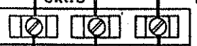
These components field mounted in control panel of unit. 460V Heater Terminal Block
