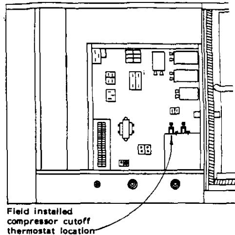
**IMPORTANT NOTE:** Only the thermostat and subbase combinations as shown above will work with this equipment. The stat and subbase MUST be matched, and correct operation can be assured only by proper selection and application of these parts.
