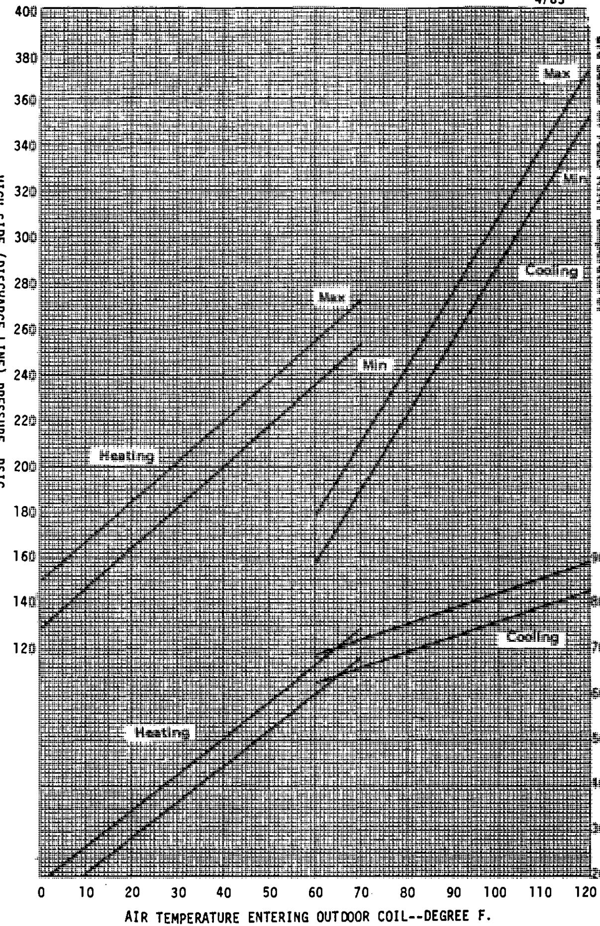
CFM (airflow) across the evaporator coil and should be used for reference purposes only. Specific information can be found under section titled "Refrigerant Charge" elsewhere in manual. If there is any doubt as to correct operating charge being in the system, the charge should be removed, system evacuated, and recharged according to serial plate instructions. Heating curves
