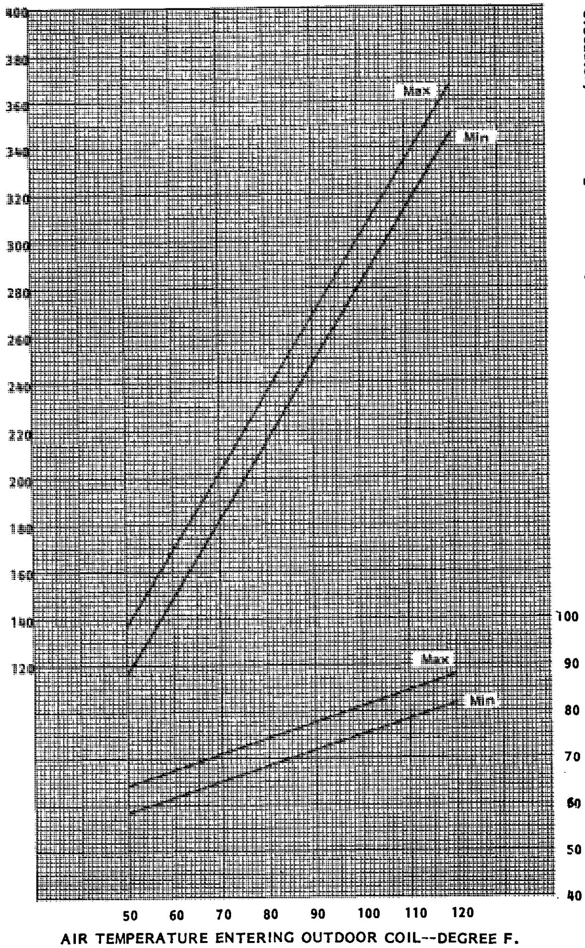
These curves are based upon 80°DB, 67°WB R.A. Temp. and rated (airflow) across the evaporator coil and should be used for reference purposes only. Special information can be found under section titled "Refrigerant Charge" elsewhere in manual. If there is any doubt as to correct operating charge being in the system, the charge should be removed, system evacuated, and recharged according to serial plate instructions.
