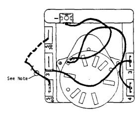
NOTE: 2 ton modal connected to 5/30 terminal (30 minutes) as shown by dotted line. Any model can be changed from 60 minutes to 30 minutes by unplugging from 5/60 terminal and reconnecting to 5/30 terminal.
