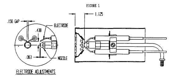
Gun Assembly Adjustment. The gun assembly can be adjusted in the slot inside of fan housing by loosening screw holding slot cover in position. Nozzle tip should ordinarily be located 1-1/8" behind the front face of the cone.
