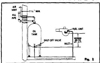
The SUNDSTRAND MODEL "A"-70 FUEL UNIT may be installed ONE-PIPE with Gravity Feed or Lift.
