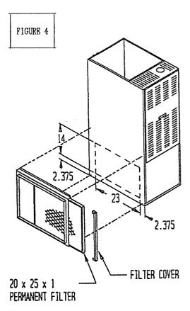
To remove filter from the filter rack, remove the filter access cover and grasp the end of the filter. This filter is the permanent high velocity type foam filter which may be washed and used over and over. DO NOT replace it with a fiberglass disposable filter of the same size.
