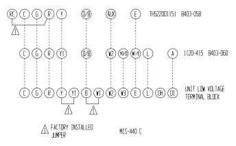
Ten (10) wires should be run from thermostat subbase to the 24V terminal board in the unit. A nine conductor, 18 gauge copper color-coded thermostat cable is recommended. The connection points are shown in Figure 8:
