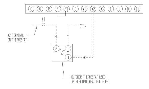
FIGURE 12 ELECTRIC HEAT HOLD-OFF WIRING 15 – 20KW 1 PH & 3 PH
