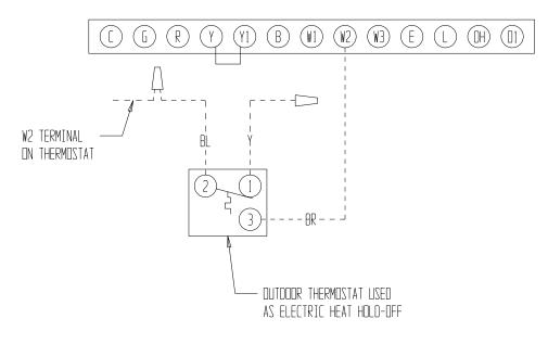
FIGURE 12 ELECTRIC HEAT HOLD-OFF WIRING 15 – 20KW 1 PH & 3 PH
