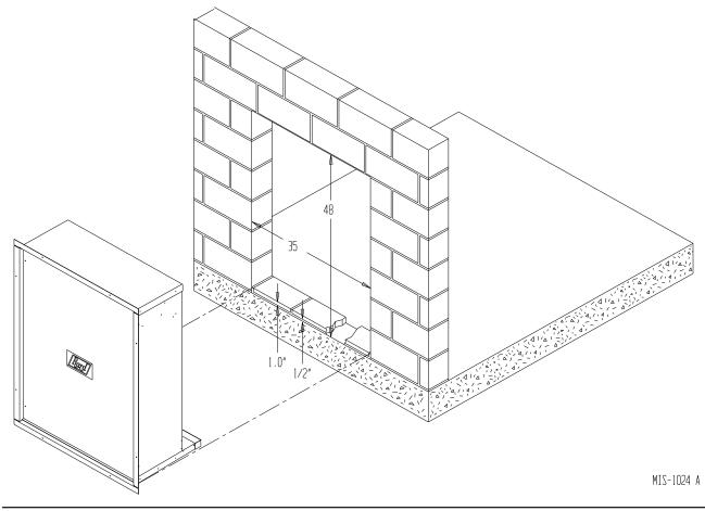
FIGURE 4 MASONRY CONSTRUCTION INSTALLATION
