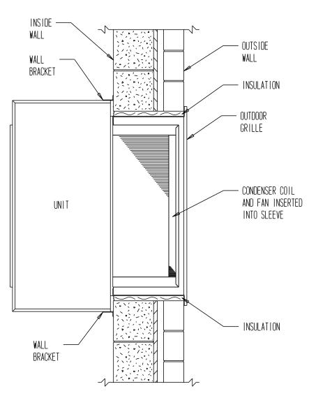
FIGURE 5 TYPICAL INSTALLATION WITH 14" MAX. WALL THICKNESS
