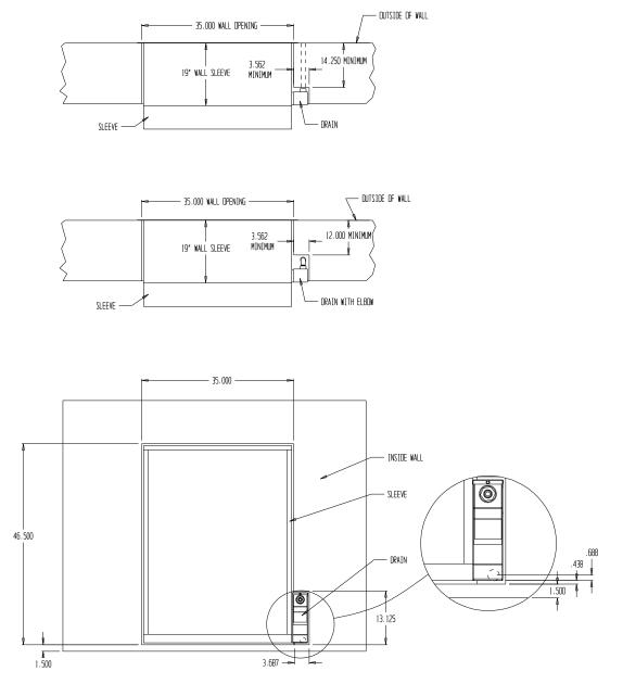
FIGURE 6 QCDS48A CONDENSATE DISPOSAL SYSTEM
