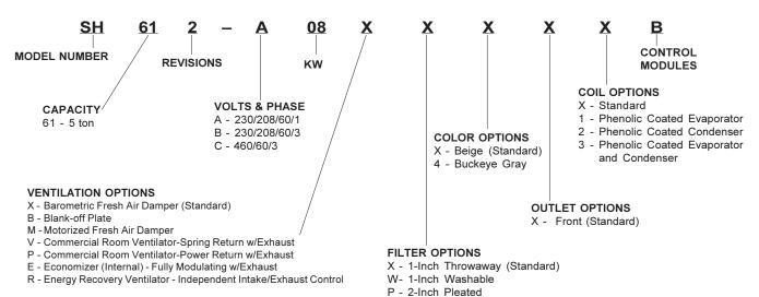
NOTE: All vent options are without exhaust capability. May require separate field supplied barometric relief in building.
