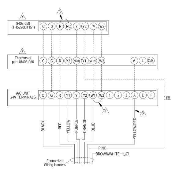
Factory installed jumper. Remove for 2-stage operation on units with 15 or more kw.
