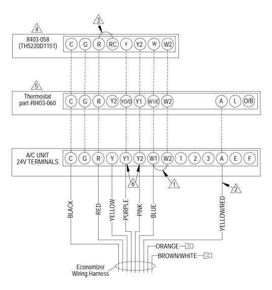
Factory installed jumper. Remove for 2-stage operation on units with 15 or more kw.
