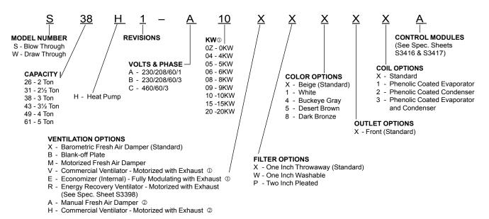
NOTE: Vent options X, B and M are without exhaust capability. May require separate field supplied barometric relief in building.
