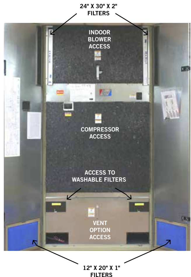
FIGURE 9 FILTER LOCATION
