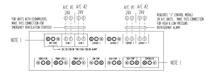
USE SHADED TERMINALS FOR DESIGNATED ALARMS AS DESIRED. SOME RELAYS ARE REVERSE ACTIVATED TO ACHIEVE "NC" OPEN-ON-ALARM SEQUENCE. EACH CAN BE USED INDIVIDUALLY IF THERE ARE ENOUGH BUILDING ALARM POINTS AVAILABLE OR CAN BE ARRANGED INTO SMALLER GROUPS OR EVEN A SINGLE GROUP SO THAT ALL ALARM CAPABILITIES CAN BE UTILIZED. FOR "NC" OPEN-ON-ALARM STRATEGY MULTIPLE ALARMS IN A GROUP ARE WIRED IN SERIES.
