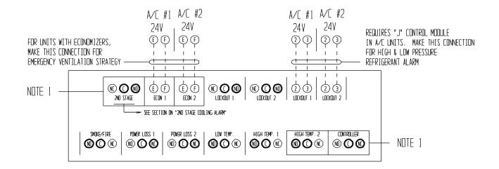
LISE SHADED TERMINALS FOR DESIGNATED ALARMS AS DESIRED. SOME RELAYS ARE REVERSE ACTIVATED TO ACHIEVE "NO" CLOSE-ON-ALARM SEQUENCE. EACH CAN BE USED INDIVIDUALLY IF THERE ARE ENDUGH BUILDING ALARM POINTS AVAILABLE OR CAN BE ARRANGED INTO SMALLER GROUPS OR EVEN A SINGLE GROUP SO THAT ALL ALARM CAPABILITIES CAN BE UTILIZED. FOR "NO" CLOSE-ON-ALARM STRATEGY MULTIPLE ALARMS IN A GROUP ARE WIRED IN PARALLEL.
