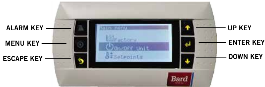
FIGURE 1.29 Bard-Link™ Controller Display
