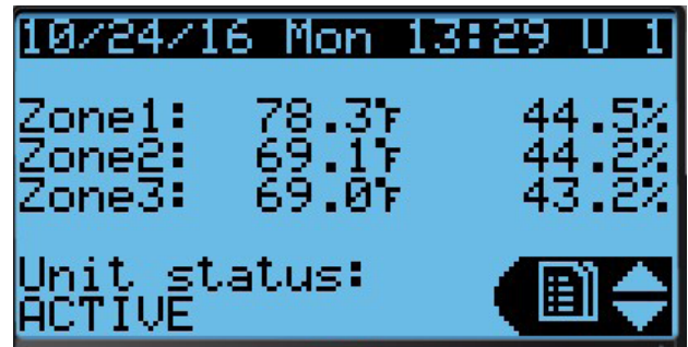
FIGURE 2.8 LC6000 Status Screen Showing Control Values
