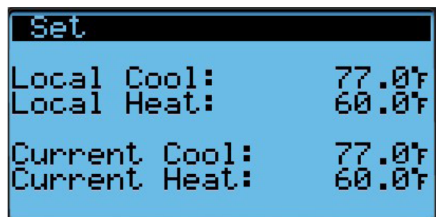
FIGURE 2.4 Local Cool/Heat and Current Cool/Heat Setpoints
