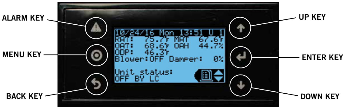
FIGURE 2.1 TEC-EYE™ (Bard P/N 8301-059) Display and Interface (Status Screen Shown)
