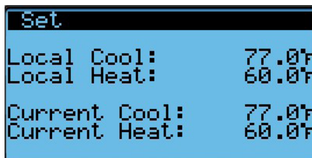
FIGURE 2.4 Local Cool/Heat and Current Cool/Heat Setpoints
