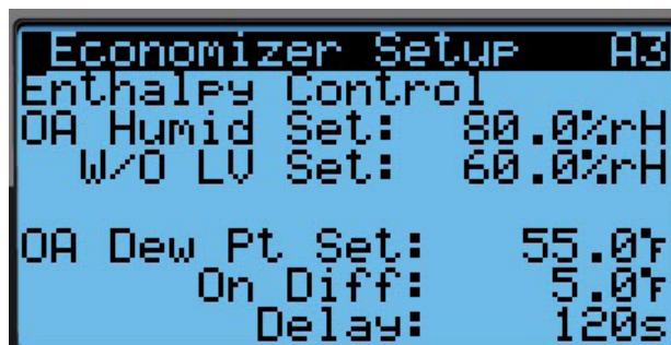
FIGURE 40 Economizer Setup – Enthalpy Control
