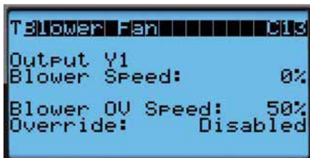
FIGURE 16 Putting Blower Output into Override Mode
