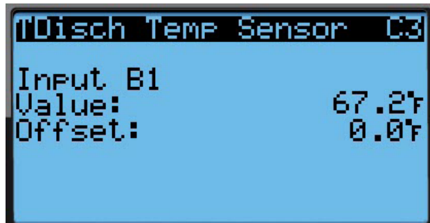
FIGURE 27 Adjusting Discharge/Liquid Temperature Input
