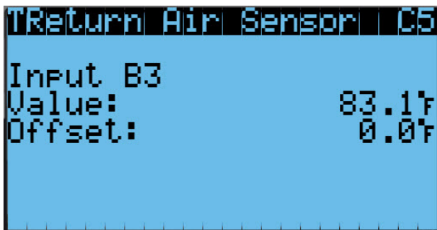
FIGURE 6 Adjusting Return Air Sensor
