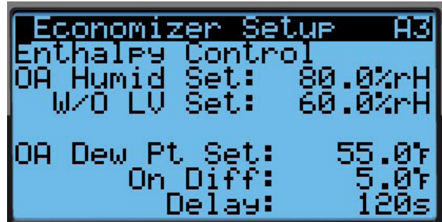
FIGURE 42 Economizer Setup – Enthalpy Control
